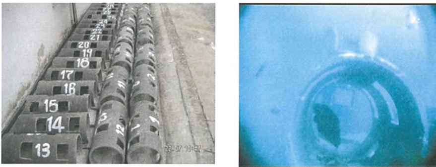
Fig. 24 Horizontal cylinder concrete tube (diameter 20cm, 60 cm long)
