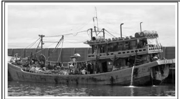
Example of a typical purse seiner fishing boat called "pekalongan" (14 – 24 meters in length and over)
