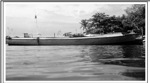
Example of a typical handline fishing boat called "sekoci sulawesi" (8 – 15 meters in length)
