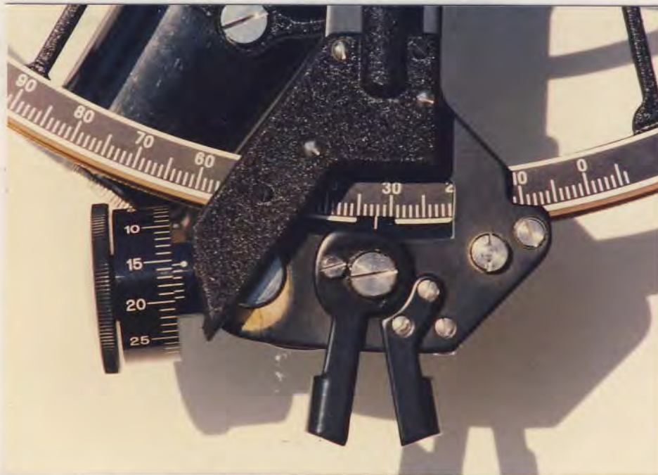
Fig. 220 The reading 32^{\circ}15'6 is the included angle between landmarks B and C.
