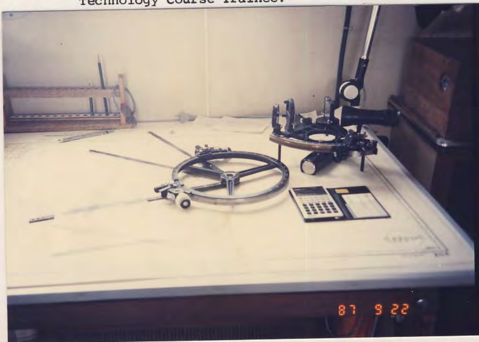
Fig. 213-4 Fix by Sextant & Three-arm protractor 22 Sept, 1987 M.V. PAKNAM
