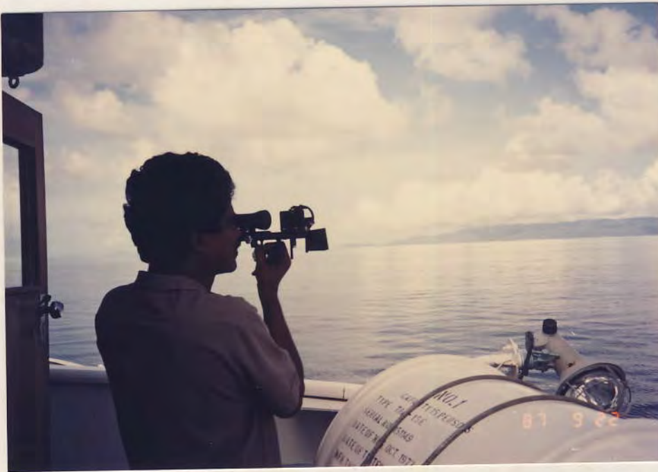
Fig. 213-3 Observing Included Angles between Samui and Phangan Island 22 Sept. 1987 M.V. PAKNAM. Observer : Mr. Krishanansamy s/o Arunasalam a 1985-1987 Fishing Technology Course Trainee.
