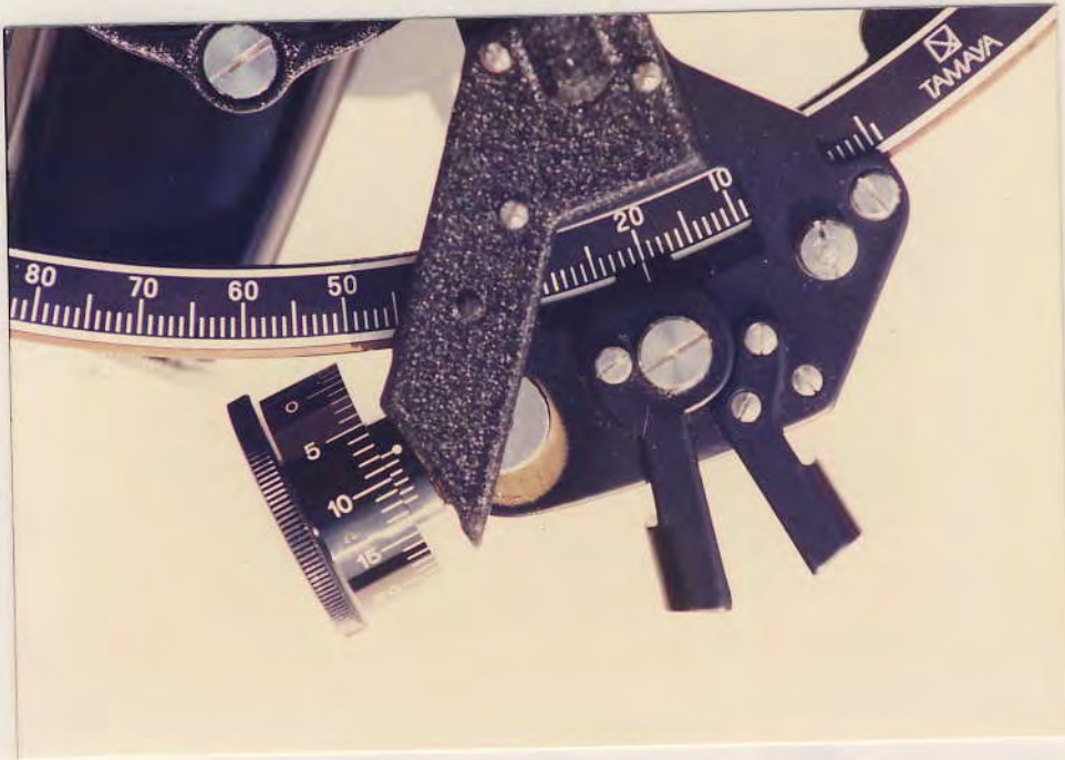
Fig. 152-2 The sextant reading is 20^{\circ} 08' 2''
