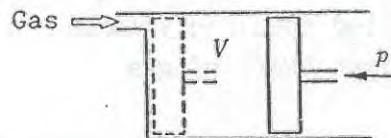
Fig. 4-2 Work done by Gas
