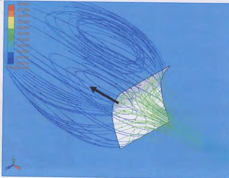
**Figure 10.** Effect of wind pressure on sail (36 m<sup>2</sup>) designed for Long tail boat
