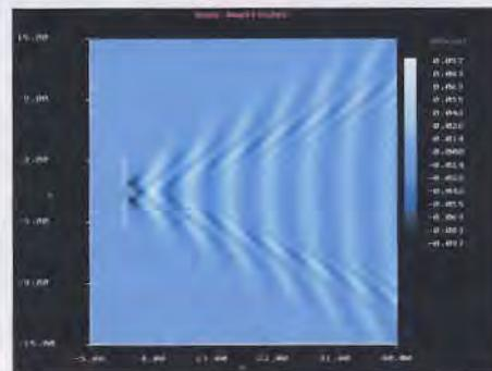
**Figure 6.** Wave-making resistance
