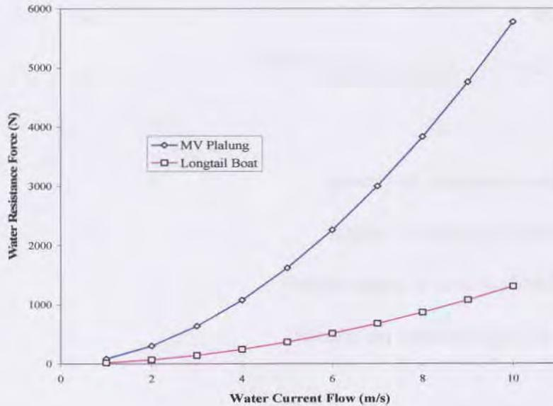
**Figure 7.** Total water resistance over hull of M.V. Plalung and Long tail boat
