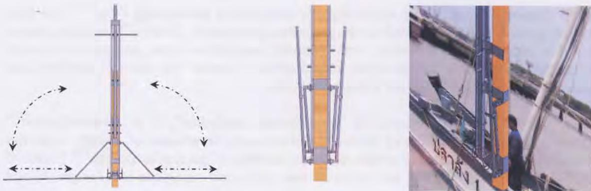
**Figure 14.** Spinnaker pole: Operation feature (left), cease-operation feature (middle), isometric view of spinnaker pole (right)
