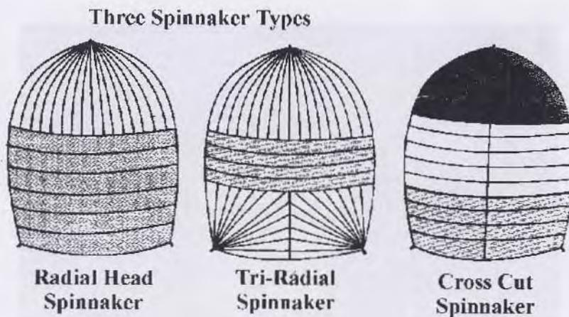
**Figure 9.** Three types of spinnaker
