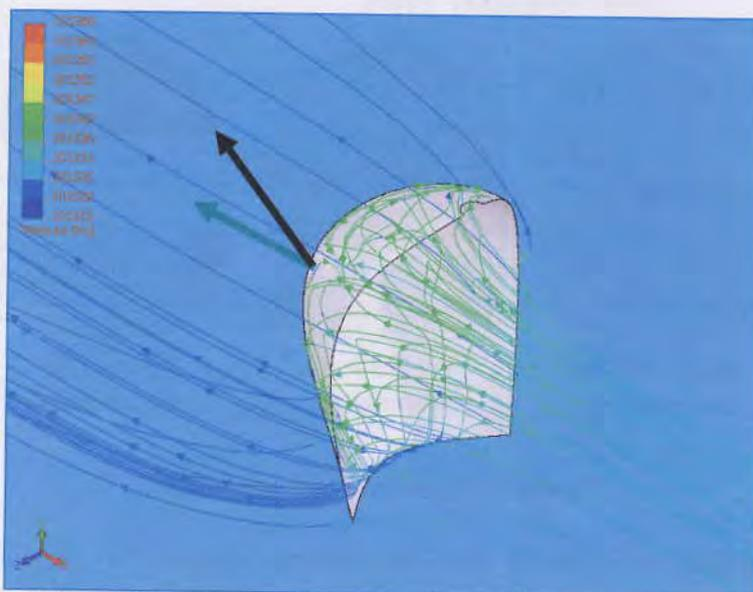
**Figure 11.** Effect of wind pressure on sail (105 m<sup>2</sup>) designed for M.V. Plalung
