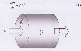
Figure. 3 Air flow through an area
