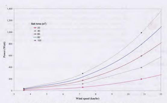
Figure 4. Relationship of the calculated wind power against wind speed
