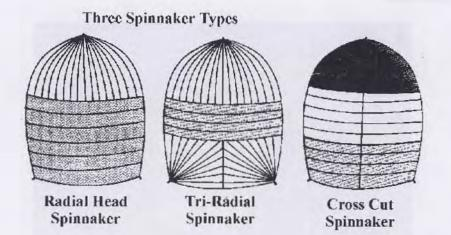
Figure 9. Three types of spinnaker
