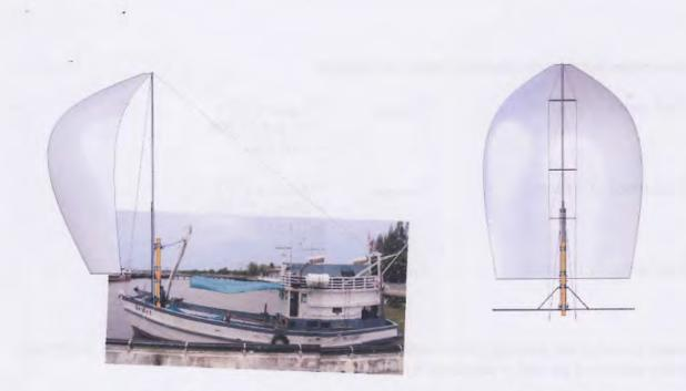
Figure 12. Right and front view of additional sail on M.V. Plalung
