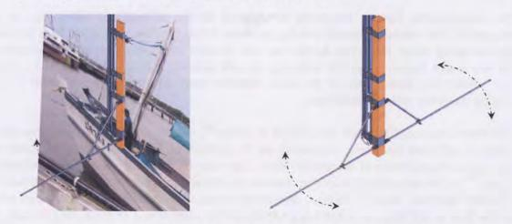
Figure 15. Isometric view of a side of spinnaker pole: Adjustable horizontal pole angle for directional control of sail
