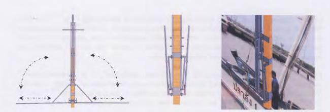
Figure 14. Spinnaker pole: Operation feature (left), cease-operation feature (middle), isometric view of spinnaker pole (right)
