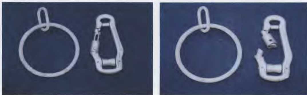
Figure 15: Right: Traditional round shape purse ring (right) and double roller purse ring (left) Left: Double roller purse ring (left) open the ring when release from purse line (Photo by Audio Visual Section, SEAFDEC/TD, 2001)
