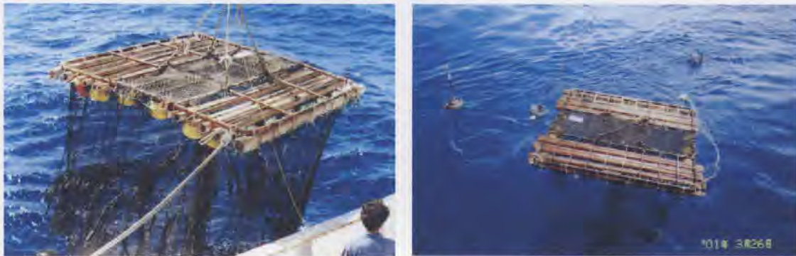
Figure 28: R/V Nippon Maru Drifting Payao Raft design
