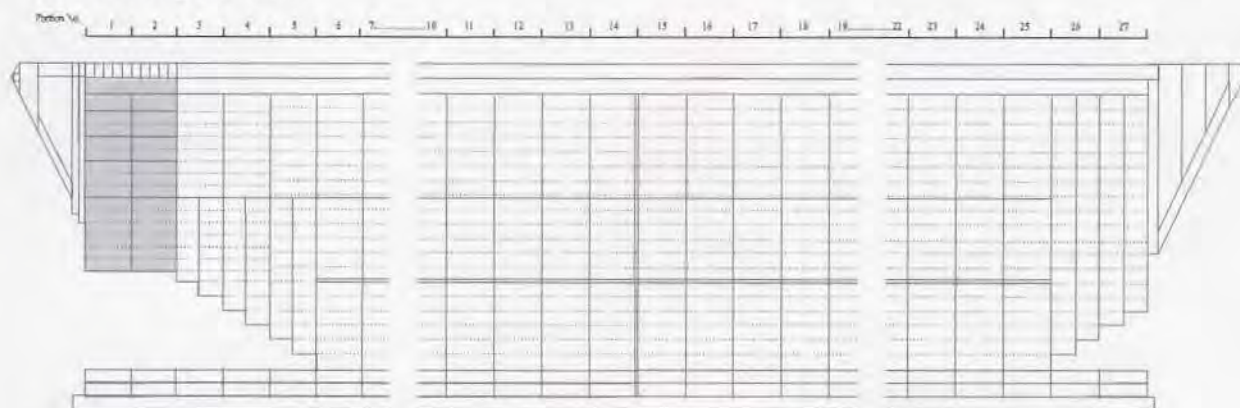
Figure 17: Bunt part (Shadow zone) of tuna purse seine net, portion No. 1 and No.2 (Illustrated by Pratakphol Prajakjitt)
