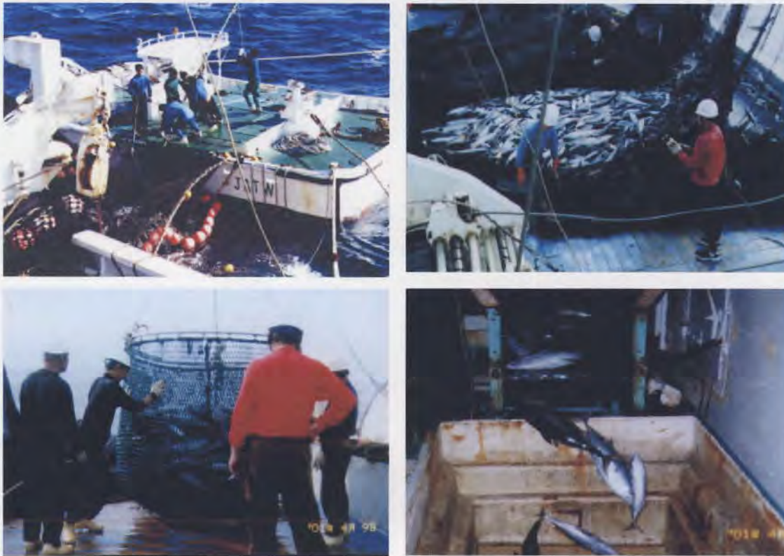
Figure 46: Activities continued by fish scooping from net to hopper and from hopper to fish dropped into fish hold through a conveyer
