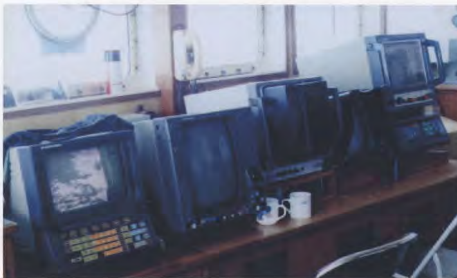
Figure 2: Navigation-aid instruments on the bridge of R/V Nippon Maru (Left to right: NOAA satellite receiver display, Navigation radar display, JRC bird radar display, Furuno bird radar display, Color plotter display)
