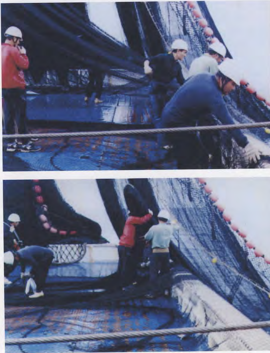
Figure 45: Bunt hauling by cargo hoists, double braid rope and crew
