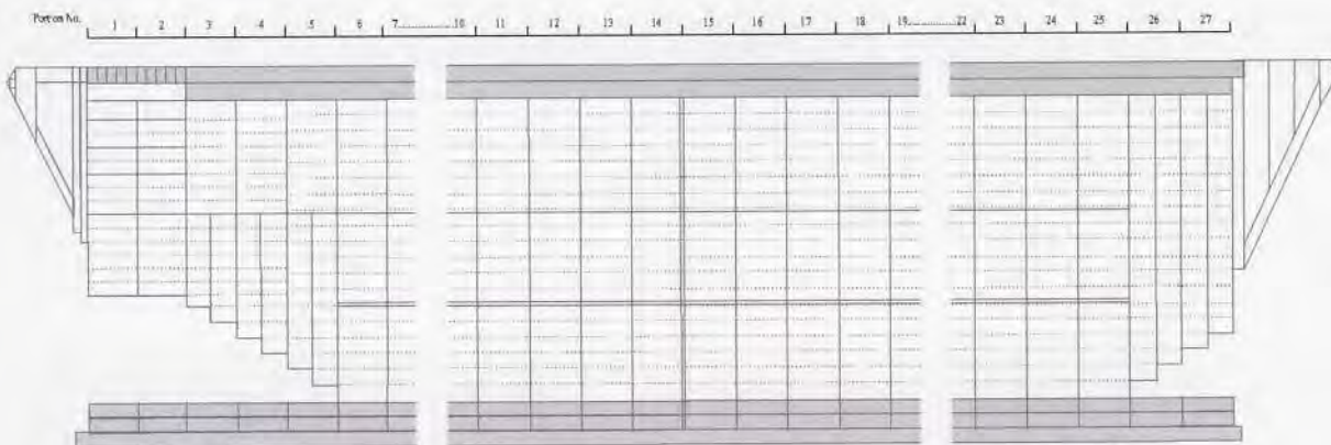
Figure 21: The location of Upper and Lower (Shadow zone) of purse seine net (Illustrated by Pratakhhol Prajakjitt)
