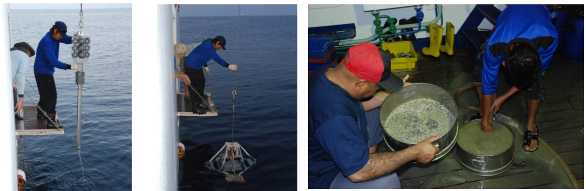
Figure 9 Sediment samplings by Bottom samplers: grab and corer
