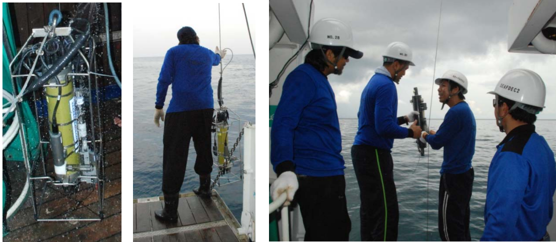
Figure 4 Oceanographic survey by CTD (Left and middle) and water sampling (right)
