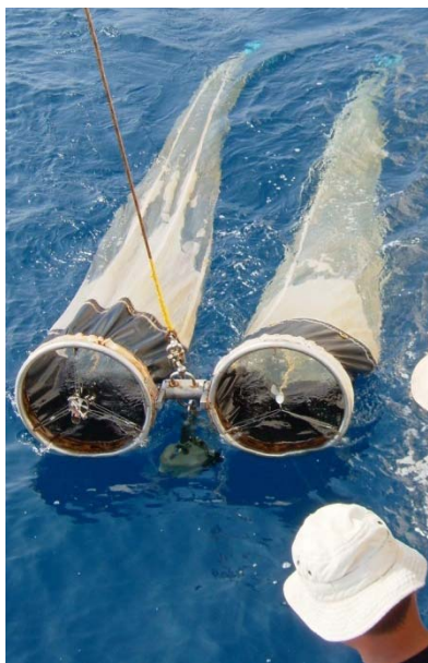
Figure 6 Zooplankton and larval fish samplings by Bongo net and sample preservation activities
