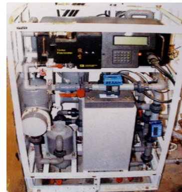
Figure 5 Thermosalinograph (TSG) & Fluorometer
