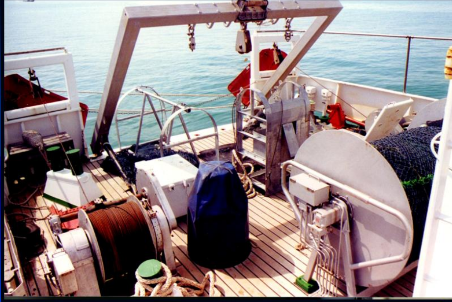
Sampling gears on deck of R/V Charkratong Tongyai Rothlisberg-Pearcy epibenthic sledge, Agassiz trawl, and Otter trawl
