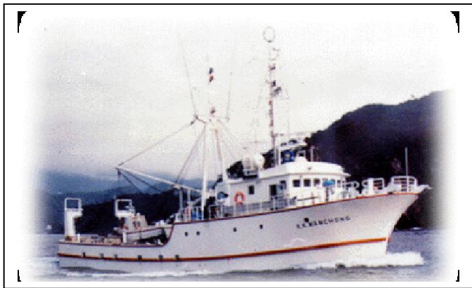
Figure 1 : Research vessel, K.K. Manchong, a stern-trawler with gross capacity of 150 GRT and powered by 90 HP engine was used during research in Malaysia EEZ water.
